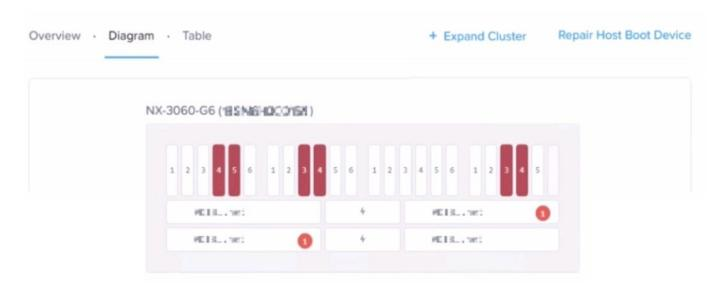
After an abrupt power outage, an administrator receives a number of alerts indicating disks are failed. Prism Element shows a large number of disks offline as seen in the diagram. This single block, four node cluster is configured FT1 with an RF2 container holding all user data.
