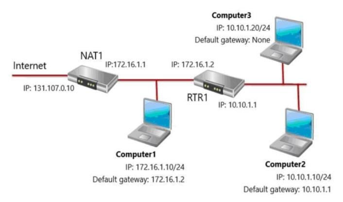
Computer1, Computer2, and Computer3 run Windows 10. Windows Defender Firewall is configured to allow ICMP traffic.
