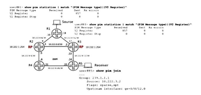
A. Configure an RP set in PIM on R1, allowing R1 to forward PIM register messages to R2 and R3 in the set.
