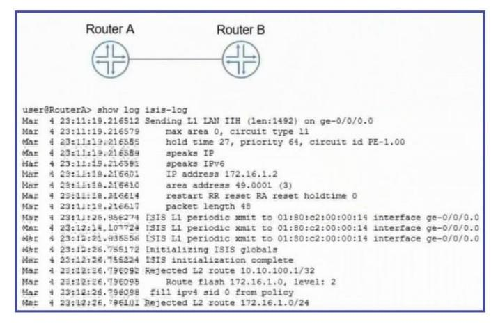
You are trying to form an IS-IS adjacency between Router A and Router B, but the IS-IS adjacency will not form between the two routers.
