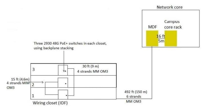
A customer needs a wired upgrade for a building on its main campus. The exhibit shows the switches that
