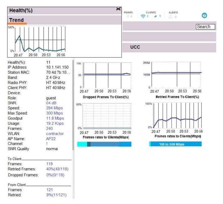
A user\\'s laptop only operates in the 2.4 GHz band and supports 802.11n. This user reports that the network is slow at the cafeteria that is serviced by three APs, and suggests that there might be a problem with the WLAN. The network administrator finds the user in the MM, and obrains the output shown in the exhibit.
