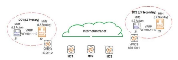
An Aruba network is deployed with L2 and L3 Mobility Master (MM) redundancy across two datacenters, as shown in the exhibit. The network administrator confirms that all Mobility Controllers (MC) are currently communicating with MM1, which is the L2 Active, and L3 Primary. Which MM IP will MCs communicate with if MM1 fails?
