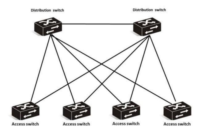
A network administrator has two distribution layer switches and four access layer switches. The network administrator is constantly resolving Spanning Tree problems and is looking for an alternative solution that provides redundancy and no Spanning Tree.
