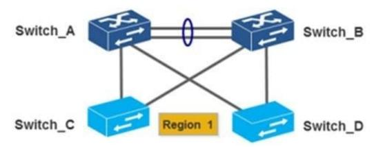
Switch\_A and Switch\_B are HP Comware switches currently in the same MSTP region with the following MSTP configuration:
