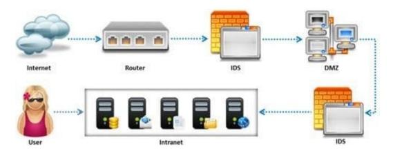
Penetration tester needs to try different combinations of TCP flags (e.g. none, SYN/FIN, SYN/RST, SYN/ FIN/ACK, SYN/RST/ACK, and All Flags) to test the IDS.
