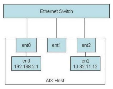
A. The ent0 and ent1 adapters must be connected to different switches to provide both additional bandwidth and adequate redundancy in the EtherChannel that is created.
