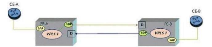
CE-A sends frames with 2 tags. If the SAP on PE-A is "sap 1/1/1:1 .\*" and the SAP on PE-B is "sap 1/1/1:100.200" how many tags will there be on the frame when it egresses from the SAP on PE-B?
