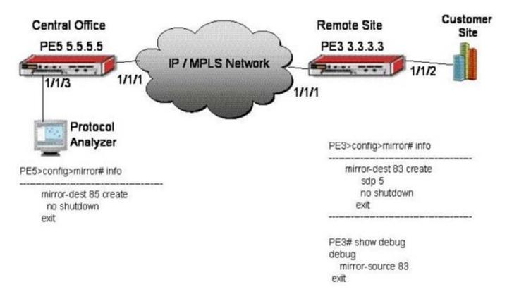
Assuming the customer only needs to monitor traffic from PE3 to the customer site, what three items are missing from PE3\\'s configuration? (Assume that the IP/MPLS network structure between the local and remote PEsis in place.) (Choose three.)
