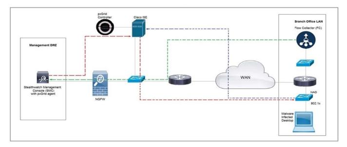
Refer to the exhibit. Cisco Rapid Threat Containment using Cisco Secure Network Analytics (Stealthwatch) and ISE detects the threat of malware-infected 802.1x authenticated endpoints and places that endpoint into a Quarantine VLAN using Adaptive Network Control policy.
