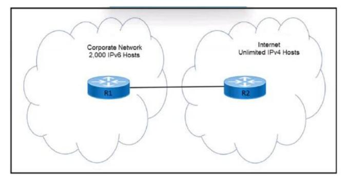
An engineer must design an address translation solution to provide Internet connectivity for the corporate network. The design Is restricted to the 172.16.168.0/22 subnet. Which solution must the engineer choose?
